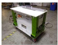
Vacuum bag and seal tabletop, or connect up to 4 tubes for your vacuum bag operation. Dual cylinder on-board vacuum pump.
