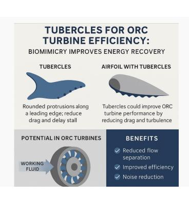
Tubercles could improve ORC turbine performance by reducing drag and turbulence
