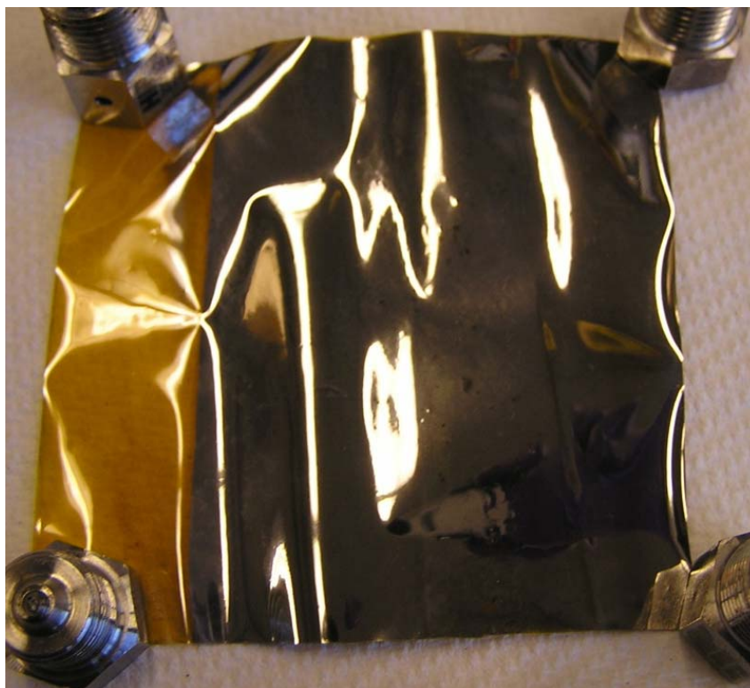
Figure 4.6: Polyamide hot wall reaction vessel liner used during experiment CoPt11. The film seen is a pure Pt flim deposited at 60 °C via SFD.
