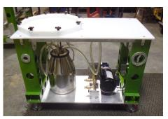
Using the Infinity Fast Filter System, expect 1L in less than 30 seconds. More wax = more time. Light wax expect 5L in less than a few minutes.
