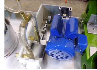
Dual cylinder on-board vacuum pump. Off-the-shelf parts means quick fix and maintenance.
