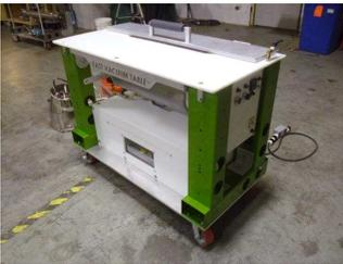
Vacuum bag and seal, or connect up to 4 tubes for your vacuum bag operation.
